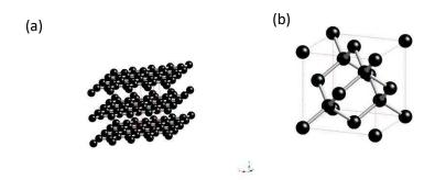
(a) Hexagonal graphite showing weak planes between the individual graphine sheets, (b) cubic diamond structure with no obvious planes of weakness.
