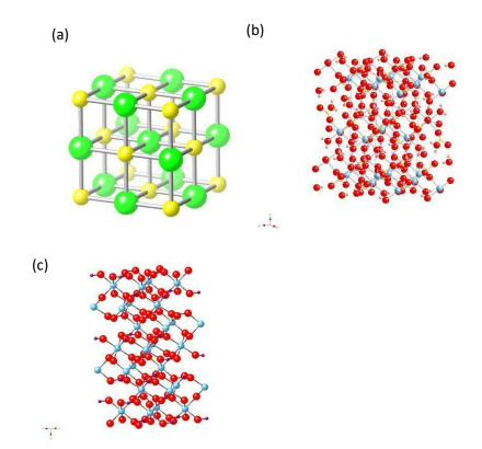
(a) Cubic halite structure showing why is breaks into cubes and (b) the more complex gypsum structures which forms angular cleavage planes which can be seen in the mineral sample. The calcite structure (c) has cleavage planes at 60/120° angles and forms more regular rhombic blocks when broken.
